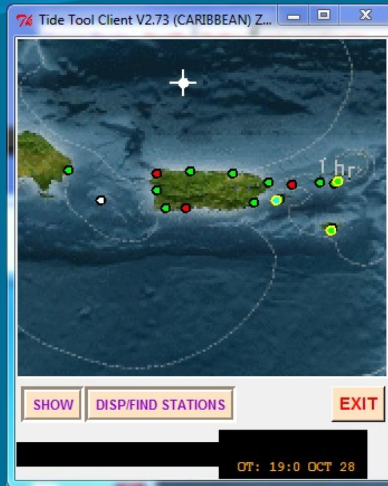
Note that the zoom widgets are larger when travel time contours are displayed. On the Client zoom widgets, the contour interval is 15 minutes. Moving the mouse over the Client zoom widget will reveal the ETA and coordinates under the cursor.
