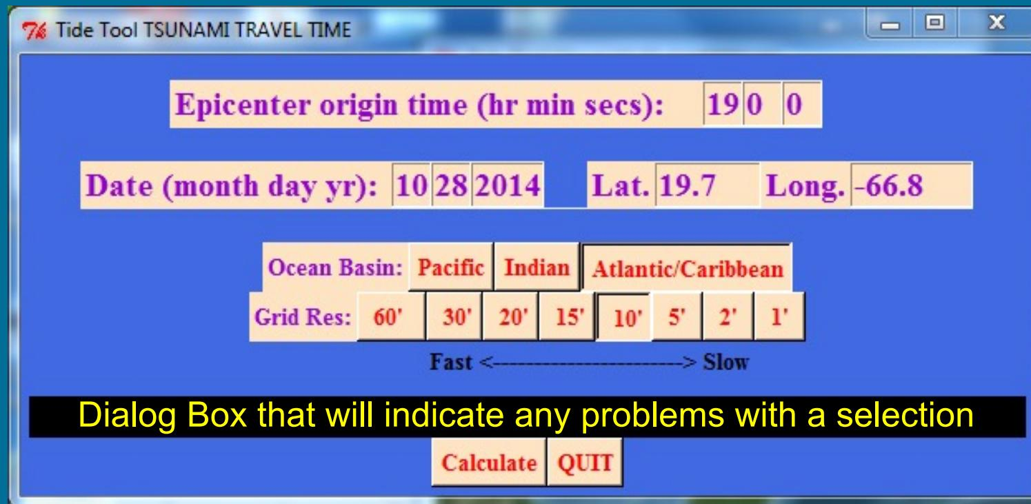
Simple to use GUI that can be invoked by hitting the TTT button on the Main GUI. A WINx cmdtool is created and the ttt\_client program is executed. When it is done...
