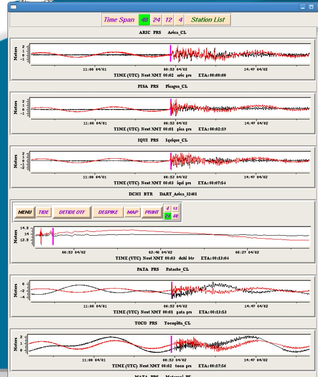
Click the “Get ETAs” button on the main GUI which loads the ETAs into Tide Tool’s data structures.
