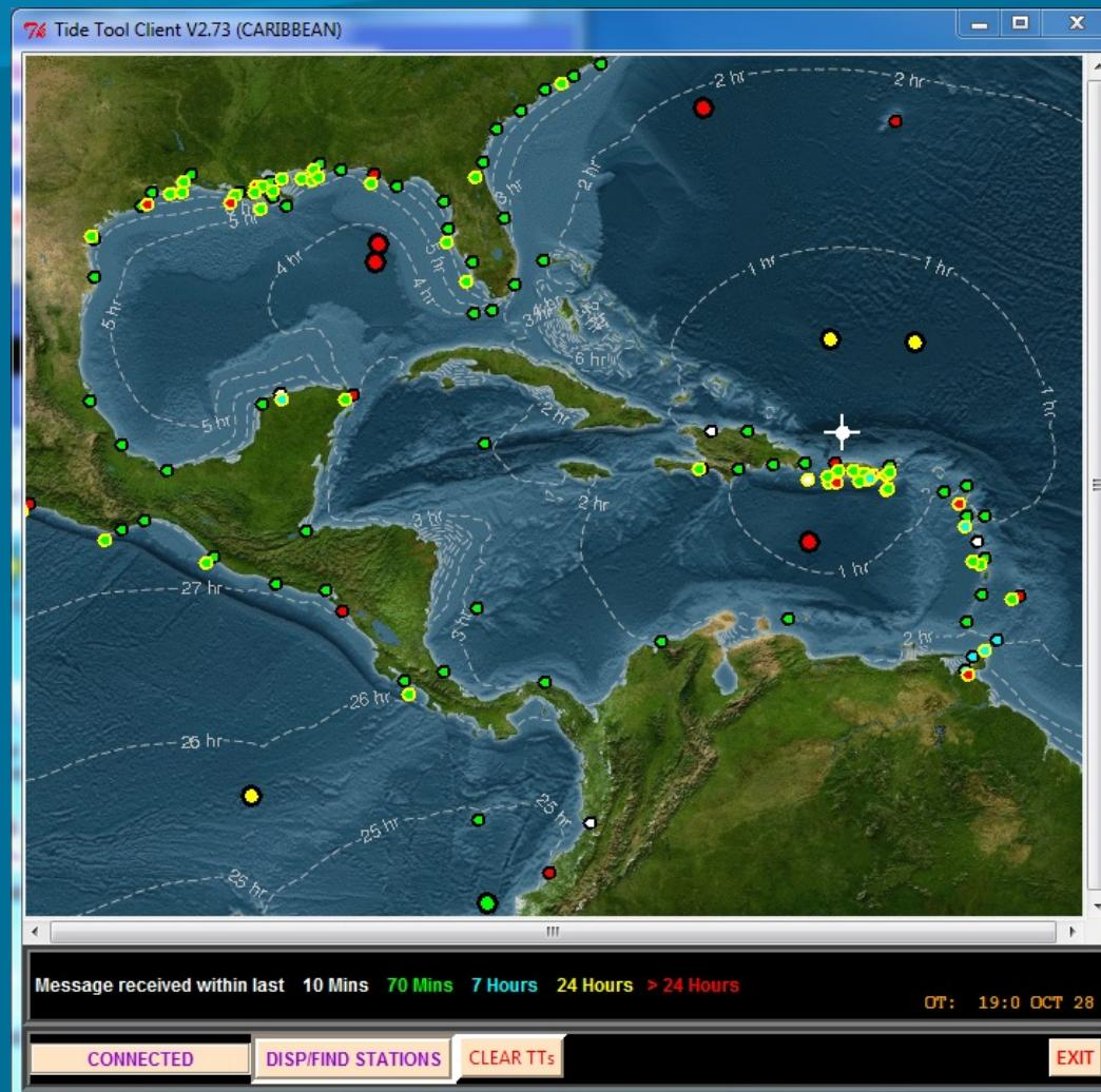
Click the “TTT” button on the base of the Client and the travel-time contours are superimposed. Moving the mouse over the Client will reveal the ETA.
