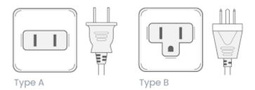
In Barbados, the standard voltage is 115V at a frequency of 50Hz. The associated plug types are Type A and Type B. Type A has two flat parallel pins, while Type B has two flat parallel pins and a grounding pin.
