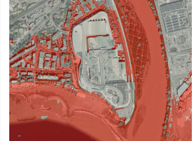
Lidar's 0-5m range extraction (in red)
